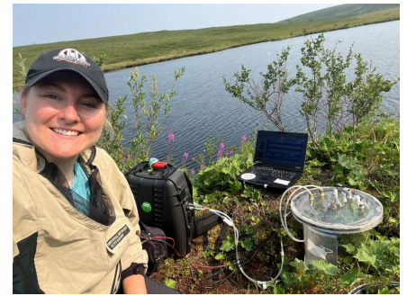
Katie measuring gas emissions from the lake. Gas collects in the clear chamber and concentrations are measured by the black analyser on the left.
